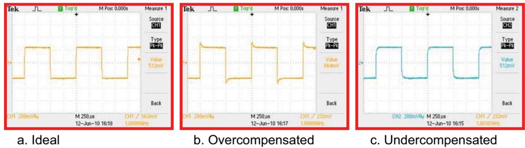
Figure 5.0-4: Measured waveforms
