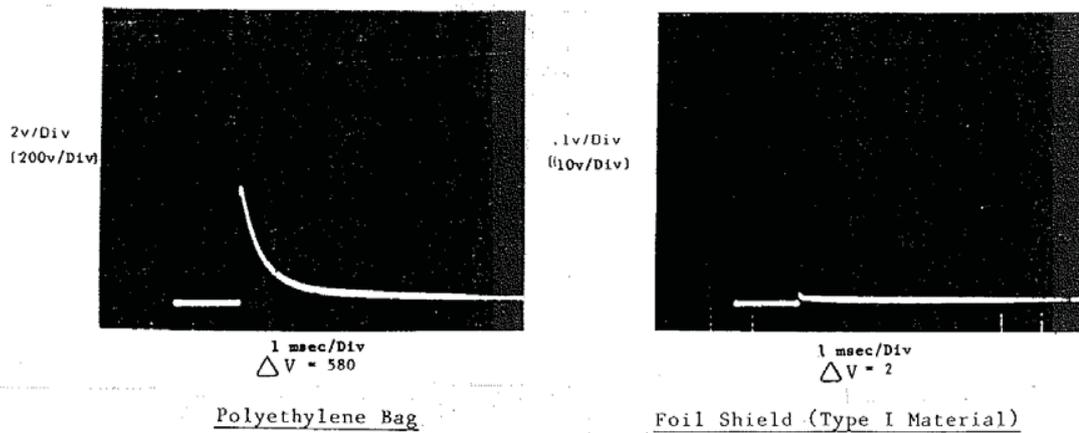
Figure 2.0-4: Voltage waveform for non-shielding and shielded bags
