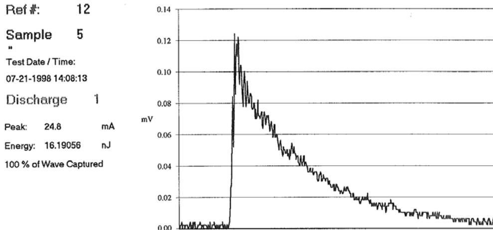
Figure 2.0-3: Typical Model 4431 shielded bag waveform
