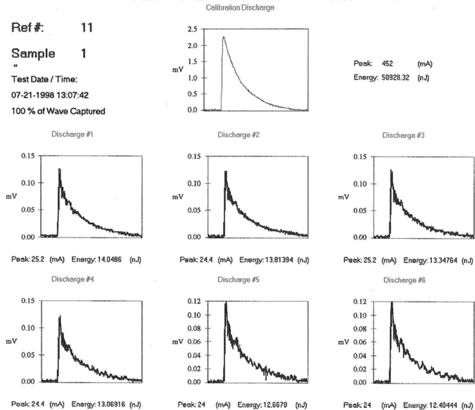
Figure 6.0-3 Typical verification and shielded bag waveforms
