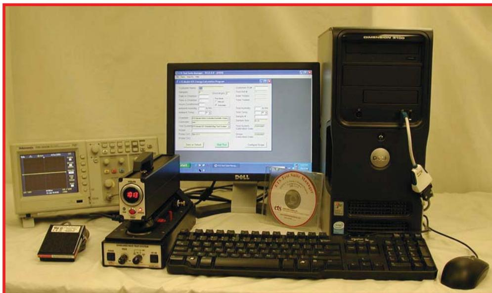
Figure 3.0-1a: Model 4431-EV Shielded Bag Test System, desktop computer
