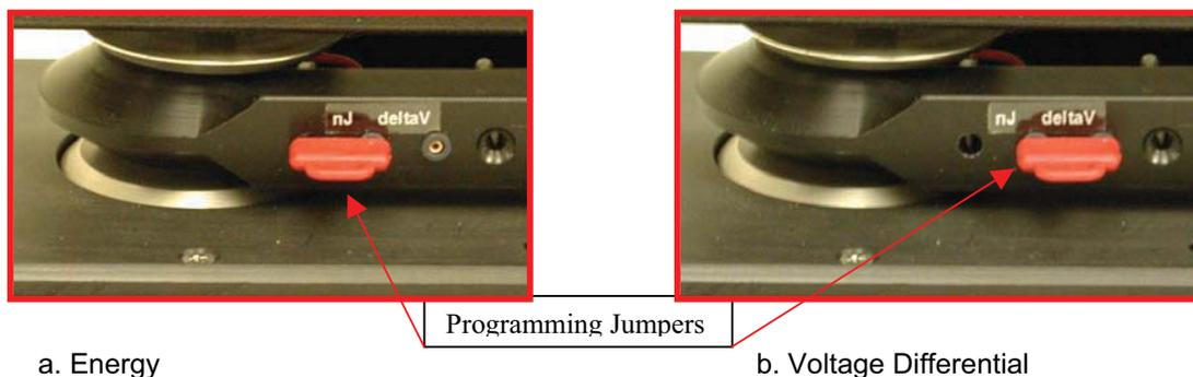
Figure 4.0-1: Capacitive sensor programming jumpers
