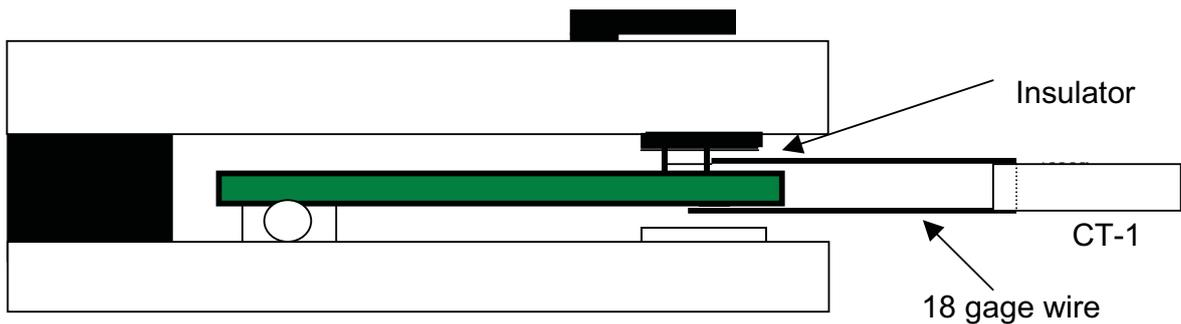
Figure 6.0-1: Calibration set up to measure ESD pulse
