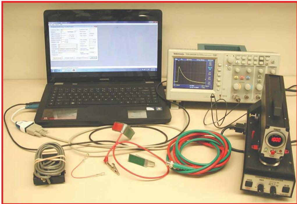
Figure 3.0-1b: Model 4431-EV Shielded Bag Test System, laptop computer
