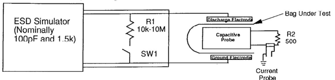
Figure 2.0-1: System generic schematic
