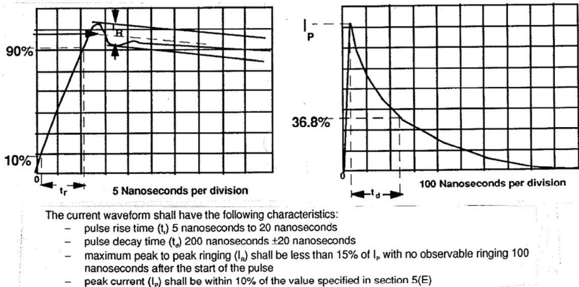
Figure 2.0-2: Discharge waveforms per ANSI/ESD STM5.1
